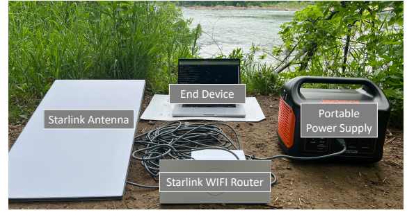
Fig. 5. StarCast Communication Test-Bed
